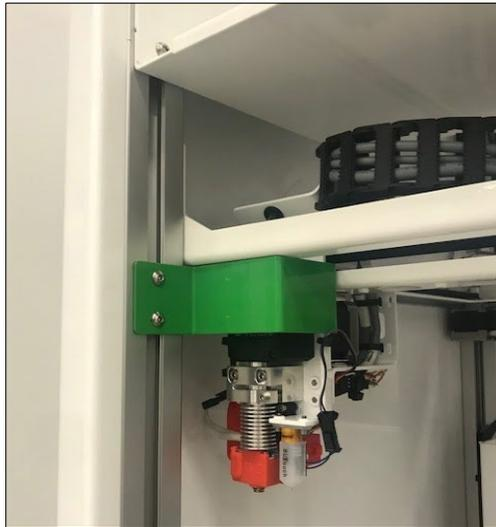
**Figure 7: Remove Bracket from Front Door**
