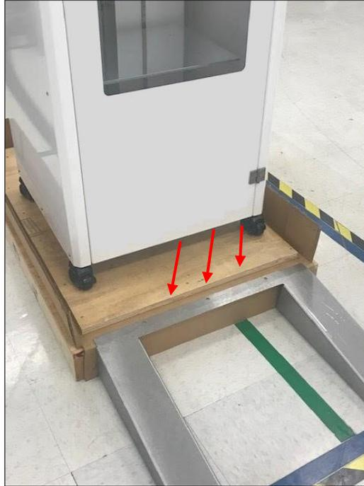
**Figure 3: Secure Metal Ramp to Wooden Pallet**
