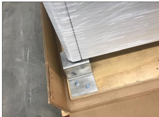
**Figure 2: Remove Metal Plates**
